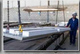
Cobute has patented an innovative system, **Panel-deck**, designed by Engineer Sandro Antonucci, to ensure fast and high-quality installation of the decking while retaining the full benefits of a **monolithic structure.**
